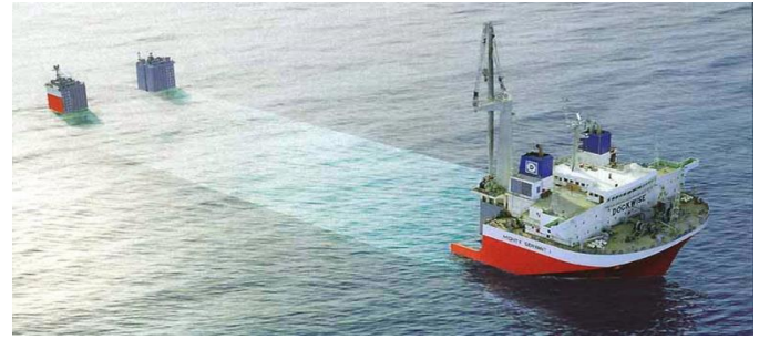
Figure 3 - Typical Float-on / Float-off Ship Ready to be Loaded.
