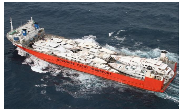
Figure 4 - Typical Float-on / Float-off Ship Fully Loaded.
